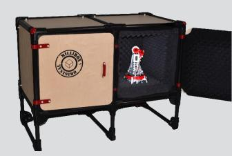
**MODULAR-** MilliBox chambers are built of modular construction components allowing the creation of several configurations to address differing needs. The MBX0x series is made of 60cm (24") cubic modules and the MBX3x series of 80cm (30") cubic modules. The chamber size is selected to satisfy your far-field requirements, and extension "cubes" can be added later if the need arises.
